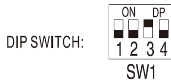
Single-phase for cooling type ( 24V Thermostat Controller)
